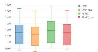
Figure 6: Hourly total cost of the different cases studied on 32 snapshots of CWE in the N-1 case. "FBMC" refers to the case of a cost-minimizing real-time model without switching. The suffix "\_rea" is for reactive switching.
