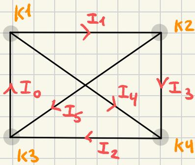
$$\begin{array}{l} K1 \quad + I_0 - I_1 \quad 0 \quad 0 \quad - I_4 \quad 0 = 0 \\ K2 \quad 0 \quad + I_1 \quad 0 \quad - I_3 \quad 0 - I_5 = 0 \\ K3 \quad - I_0 \quad 0 \quad + I_2 \quad 0 \quad 0 \quad + I_5 = 0 \\ K4 \quad 0 \quad 0 \quad - I_2 \quad + I_3 \quad + I_4 \quad 0 = 0 \end{array}$$
