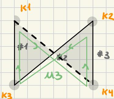
$$\begin{aligned} \mu_1^* &+ 0 - R_2 I_2 - R_3 I_3 + 0 + R_5 I_5 = 0 \\ \mu_2^* &- R_1 I_1 + 0 + 0 + 0 - R_5 I_5 = u_0 \\ \mu_3^* &+ 0 + 0 - R_3 I_3 + R_4 I_4 + R_5 I_5 = u_0 \end{aligned}$$
