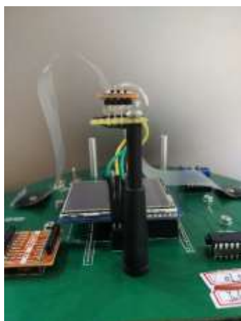
Figure 2. Compass sensor on top a tower
