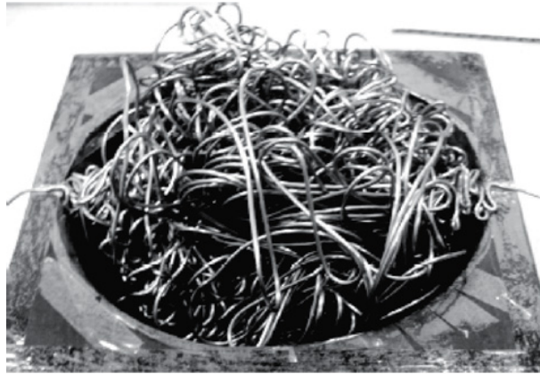
Figure 6.3: Three-dimensional packing of a ductile wire in a rigid sphere. The wire is made of a tin/lead alloy and was fed from opposite sides into a rigid hollow sphere of size q = 50 , of which only the lower half is pictured. Photograph from ref. [72], published under a Creative Commons license CC BY-NC.
