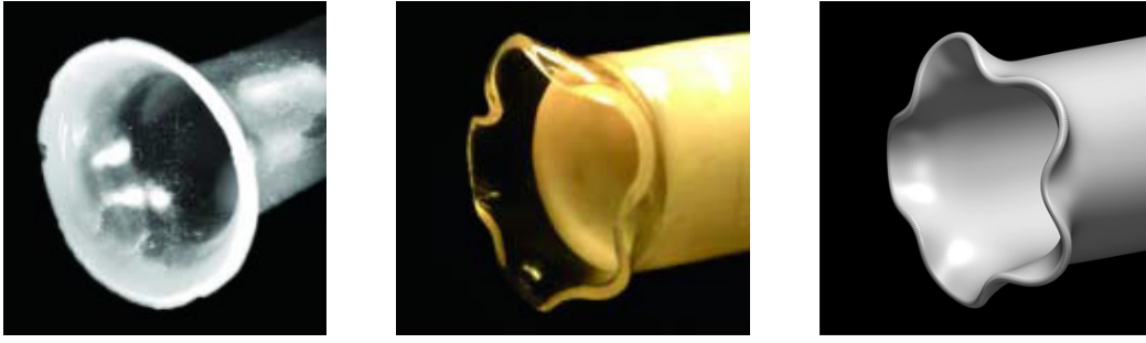
Figure 4.5: Boundary instability of a swollen gel cylinder. Left and middle: Dipping polyacrylamide gel tubes into water grows their metric profile. If the immersion depth is confined to a narrow boundary layer (short l , large metric gradient), the continuous axisymmetry is broken into a discrete one. Photographs courtesy of E. SHARON, M. MARDER and H. L. SWINNEY, reproduced from ref. [196]. Right: Computer simulation with differential growth of the form of equation (4.8).
