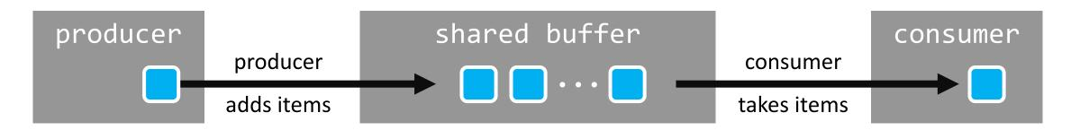
For simplicity, buffer is unbounded (has no capacity limit); producing is always possible
